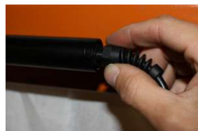
Tighten carefully by hand to make waterproof
