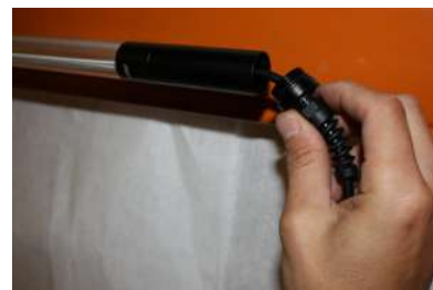
Tighten carefully by hand to make waterproof
